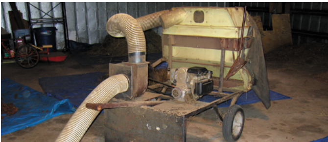
This home-made "hammermill" was created from parts of an old riding lawnmower. Essentially, the seeds are sucked through a tube, beat up by the steel fan blades, and deposited in a hopper. The process knocks seeds out of pods and off of stems.
