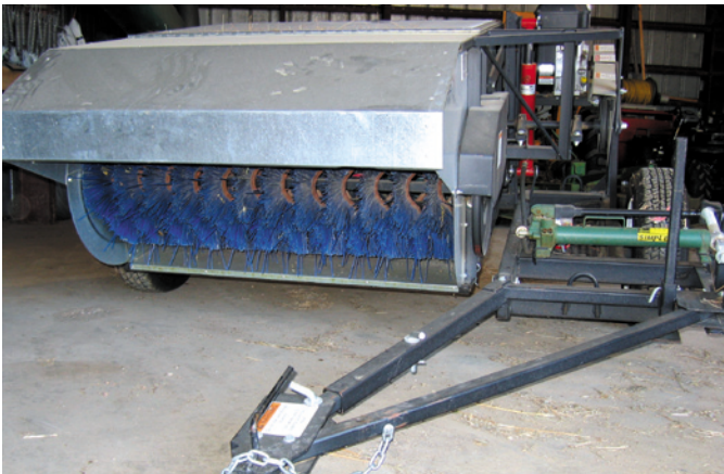
A seed stripper that can be pulled behind an ATV. The brush strips seeds into the hopper behind it.
